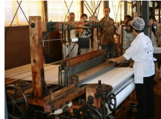
Demonstrating a wooden silk weaving machine ③
